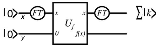
**Figure 10.** Quantum network for Shor's period-finding algorithm. Here each horizontal line is a quantum register rather than a single qubit. The circles at the left represent the preparation of the input state  $|0\rangle$ . The encircled  $ft$  represents the Fourier transform (see text), and the box linking the two registers represents a network to perform  $U_f$ . The algorithm finishes with a measurement of the  $x$  register.
